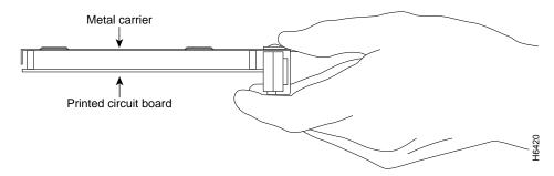
Step 6 Place the port adapter on an antistatic surface with its components facing upward, or in a static shielding bag. If the port adapter will be returned to the factory, immediately place it in a static shielding bag.
